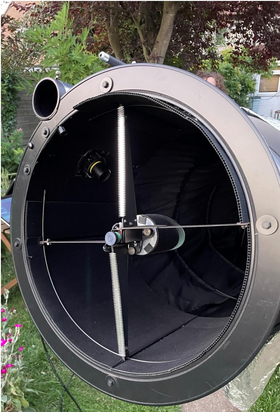
Figure 18. Apodising mask consisting of a 30° saw-tooth on 3mm pitch and attached to the two offending vanes of 444mm scope
