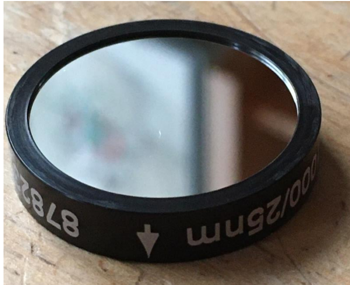
Figure 1. Edmunds Optics 1000nm filter with 25nm bandpass (Edmund Optics part number #87-823)
