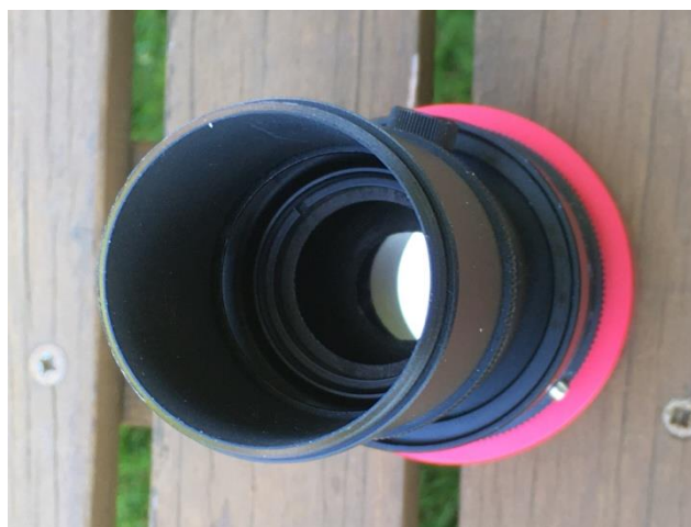
Figure 2. Custom baffled tube on front of camera with 1000nm filter half way down
