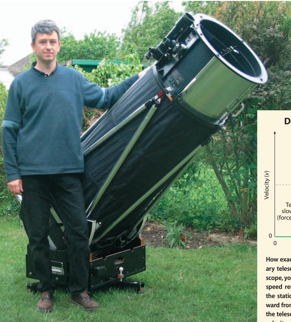
The author is seen here with "Fossil Light," his 18-inch truss-tube Dobsonian reflector. The telescope not only gives satisfying views of the night sky but also functions as a final real-world test bed for new bearing materials. All photographs courtesy the author.
