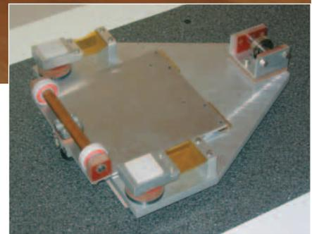
This view shows the underside of the test sled. The two white squares are test pads of perfluoroalkoxy fluorocarbon, or PFA.
