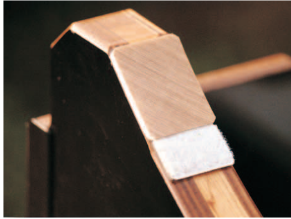
One of the altitude bearing pads using Teflon Sheet. Lewis discovered that this low-cost material performs much better than ordinary Teflon. The strip of fuzzy Velcro below acts as a dust wiper to keep the bearing surfaces clean.
