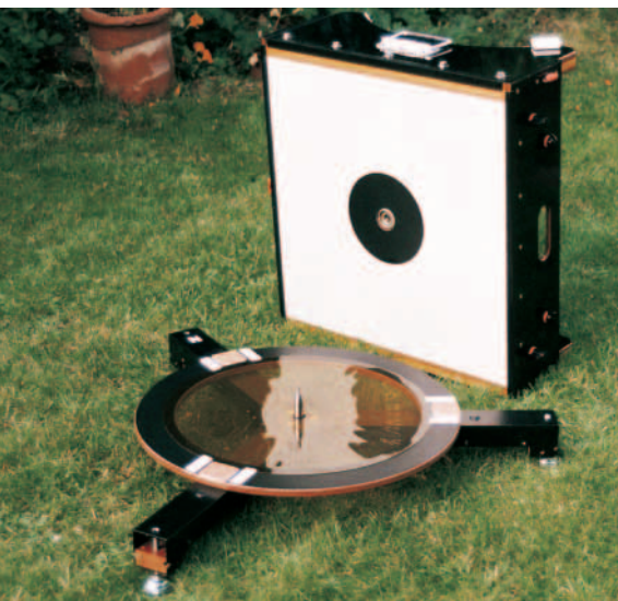
The lightweight ground board of the author's Dobsonian features adjustable feet and, of course, bearings using Teflon Sheet. These three pads bear against the bottom of the rocker box, which is faced with a textured Formica.
